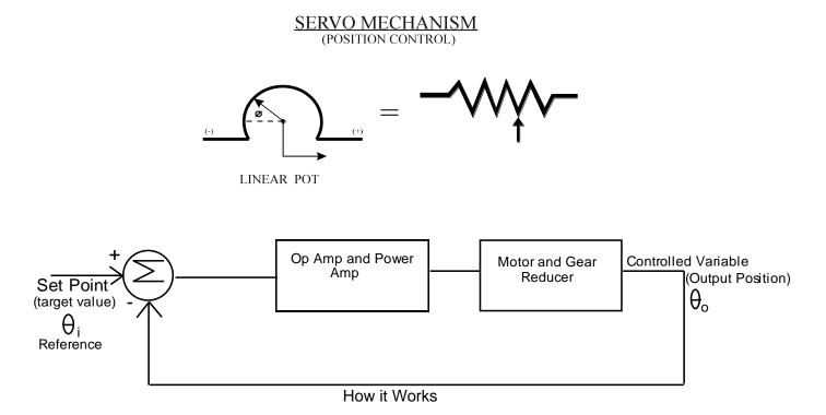
The error which is the voltage difference between the reference and the actual position produces a voltage which drives the motor in a direction that the coupled output potentiometer produces a voltage resulting in a reduced error. When the error is zero, there is no voltage to drive the motor.
