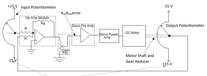
Notice the reversal of polarities of the potentiometer power supply
