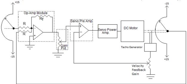
The output of the tachometer is a DC voltage that is proportional to the angular velocity of the DC motor. That is the faster the motor rotates, the greater the output from the tachometer.
