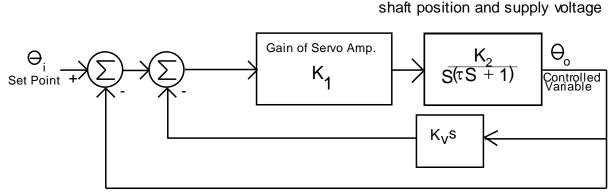
Find the transfer function of the position control system with velocity feedback.  $\kappa \kappa$
