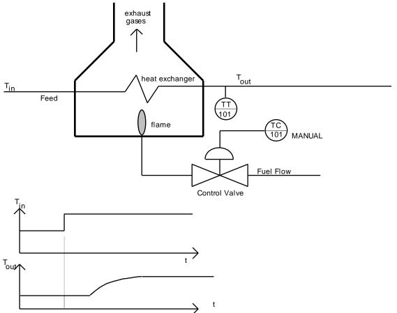
The response above is an illustration of the change of outlet temperature when inlet temperature suddenly rises. Outlet temperature rises in a first order manner after a delay (dead time). The change in inlet temperature is a disturbance. The above graph assumes that the fuel flow and feed rate is fixed. That is , no closed feedback control is employed. Below is a block diagram for the process disturbance.
