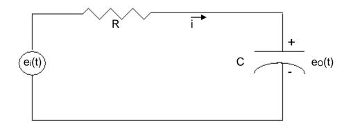
Then for the RC circuit above,  $v_{\rm C}=e_{\rm O}(t)$  , e is a function of time
